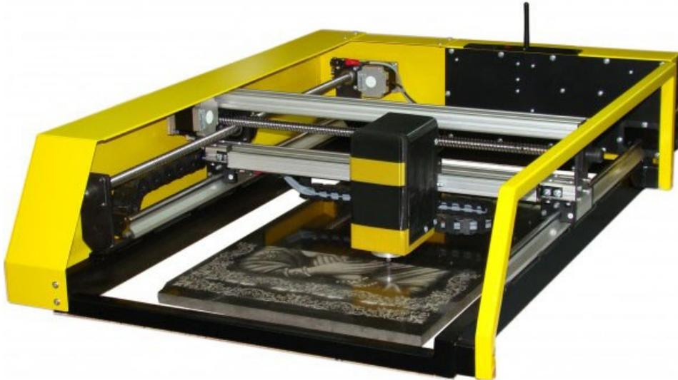
The new diamond etching machine is not a laser engraving system, it has been specifically designed to etch highly detailed ornamentation direct onto headstones. Unlike laser engraving machines the diamond etching machine does not require the stone to be level, flat or black!
